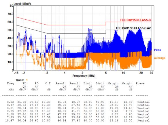
Remarks: 1. C.F (Correction Factor) = Insertion loss + Cable loss
