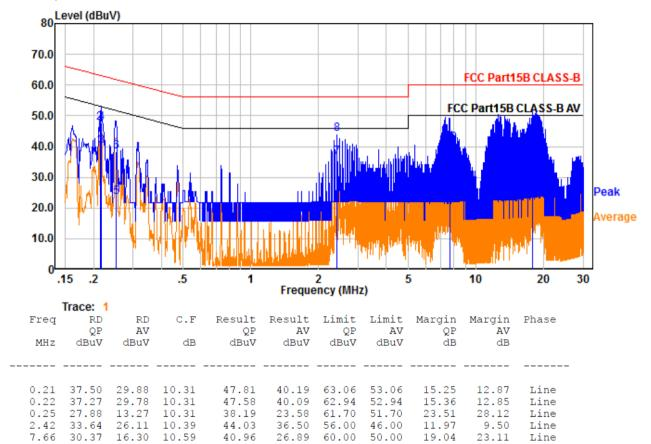
Remarks: 1. C.F (Correction Factor) = Insertion loss + Cable loss
